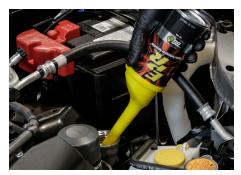
**BG EPR**<sup>®</sup> is added prior to oil change, dissolves deposits, and is removed with the used oil.
